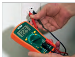
Displays AC Voltage of an outlet receptacle
